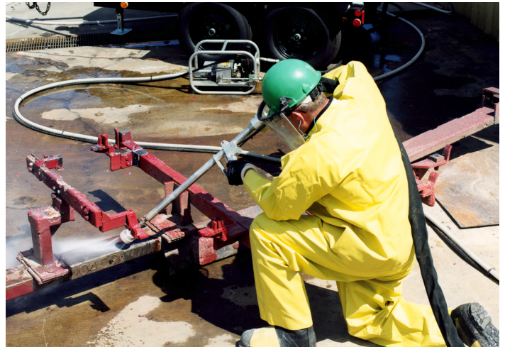
Paint removal for automotive skids using the NLB Model NCG8450A-3 rotating hand lance.
